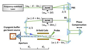
FIG. 2. Proposed experimental design for producing Doppershifted bichromatic field, compensating the phase-difference changes, and producing cryogenic molecular beam with a buffer gas beam source. The expressions labeled within parentheses indicate the laser frequencies after stabilization by some frequency-stabilization method or modulation by the acousto-optic modulators.
