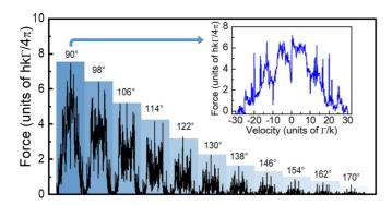
FIG. 1. The calculated relationships between the BCF exerted on YbF molecules and molecular velocities under different phase differences  $(\varphi)$  of the counterpropagating beat note envelopes from  $90^{\circ}$  to  $170^{\circ}$ . The inset shows the optimal BCF effects with  $\varphi=\pi/2$ . All the numerical solutions are calculated based on the time-dependent density matrix for 16 levels, with a 20-G magnetic field with a skewed angle of  $60^{\circ}$ .
